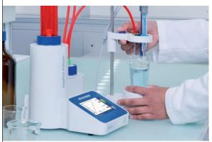
This instrument has been specifically designed to simplify the determination of sodium in food products using the standard addition technique. Simply add a sample and ionic strength adjustment (ISA) solution and start the measurement. That's it! No system calibration is necessary. Specific sodium analysis has never been so quick and easy.
